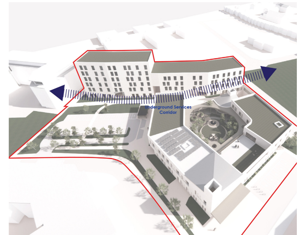
Fig. 26. Diagram indicating proposed underground services corridor
