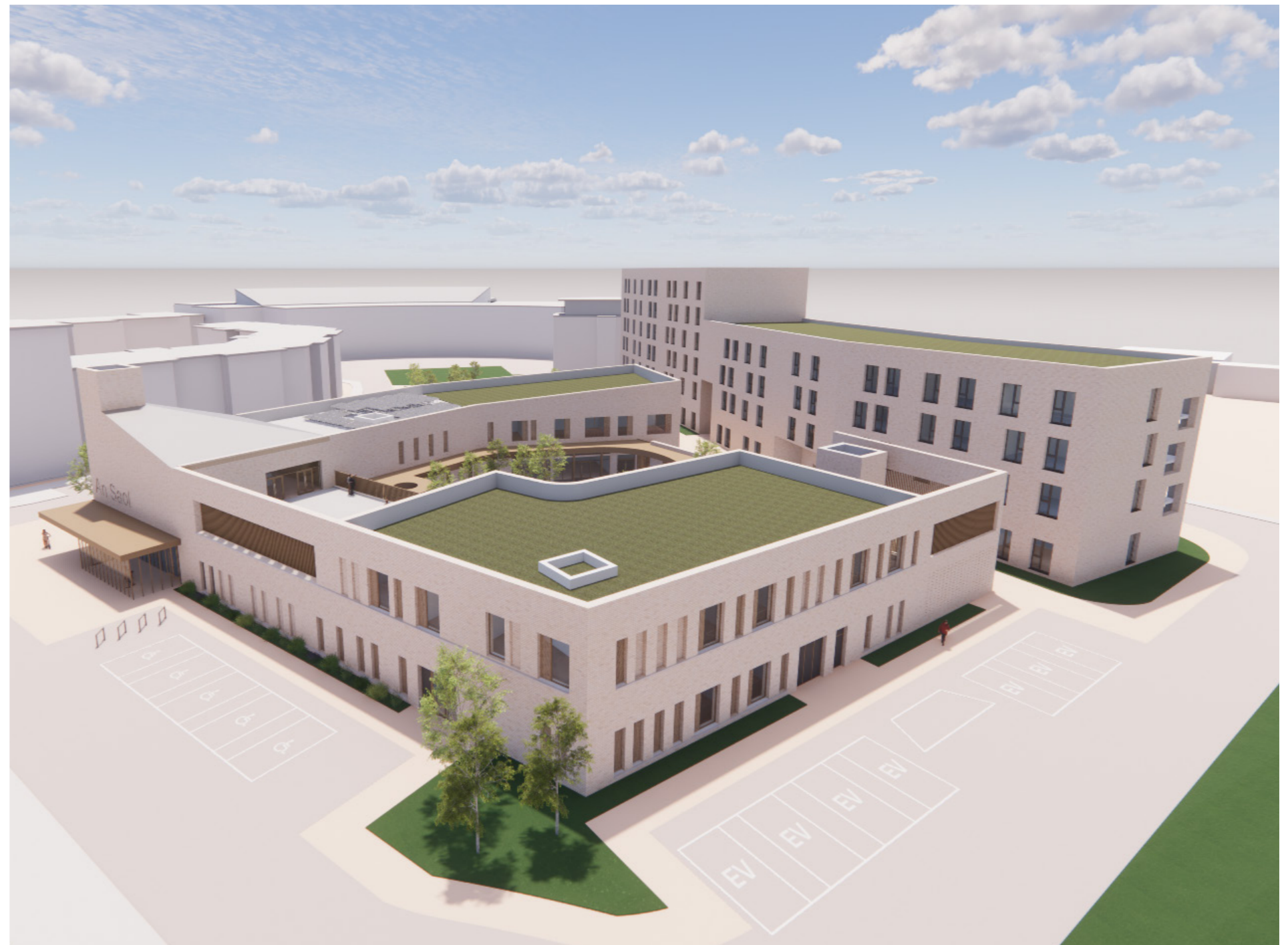
Fig: 44. 3D View of Proposal indicating Green/ Blue Roofs and Renewable Energy Solar PV's at Roof level
